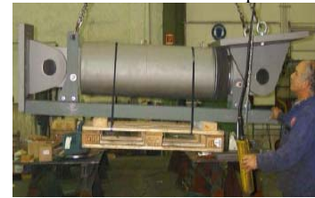
Fig. 33 A 2,500 kN MSTL for the railway viaduct De La Rambla, Spain
